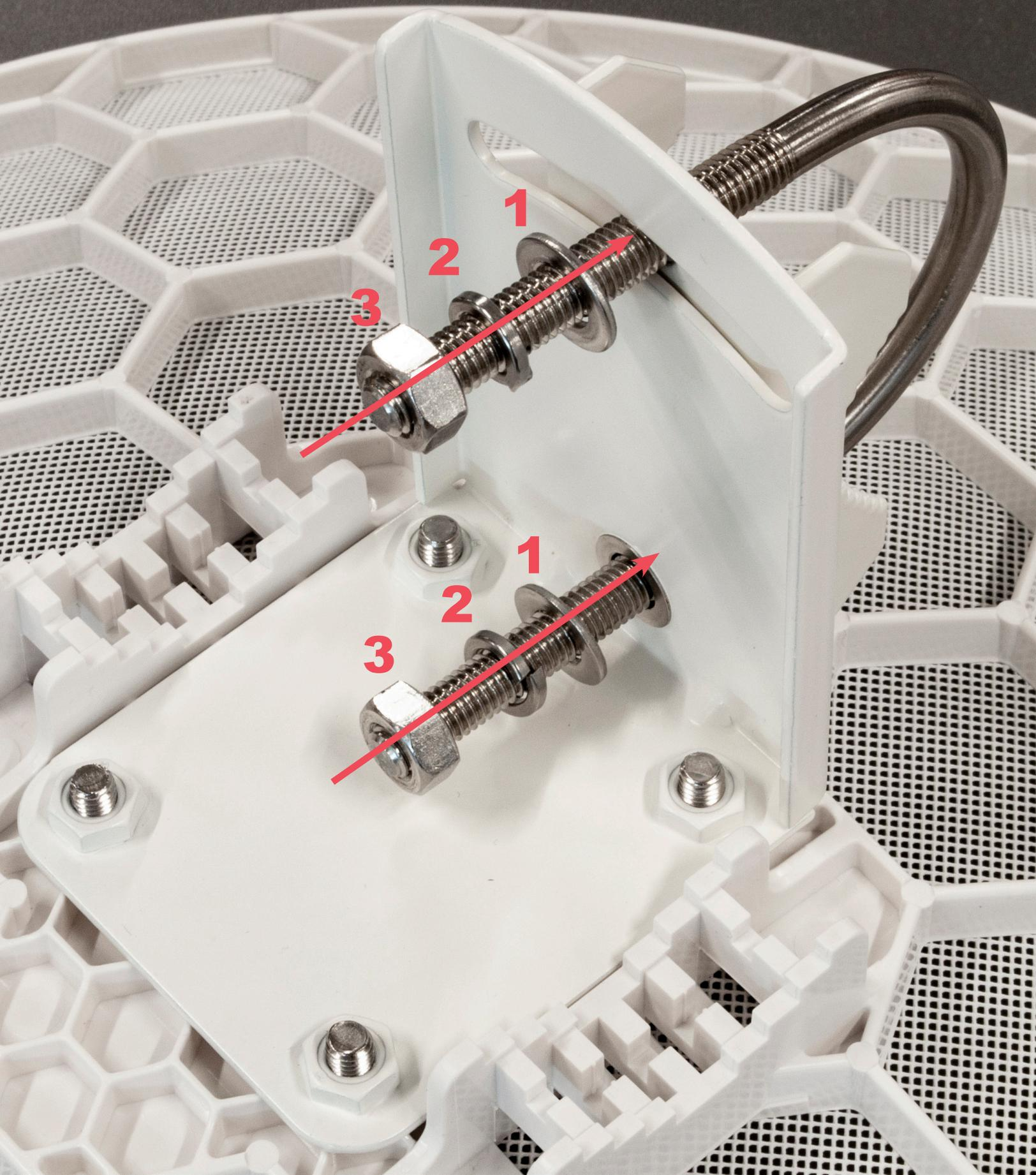
**5** Use the provided M8 washers and nuts in the order that is specified in the image. Tighten the nuts with the 1/2 wrench.
