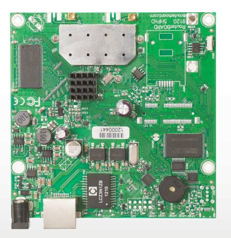
The RB911 is a small wireless router with an integrated high power wireless card. The Gigabit port helps to utilize the full potential of 802.11n wireless speeds.
